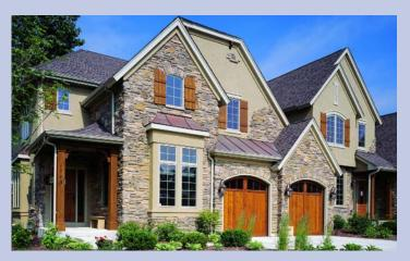
Fig. 6. Fire safety: the façade of this residence combines two noncombustible finishes, portland cement plaster (stucco) and manufactured stone veneer products, for an attractive appearance. These products are frequently made with white cement.
